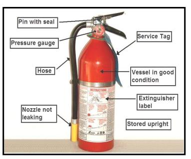
**Nozzle** – there should be no powder present on the nozzle, as this would indicate a possible leak in the valve.
