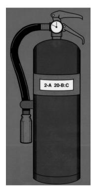
**1 unit of class A** = 5 litres of water. For example if you find a 3-A rating on your extinguisher it has an equivalent rating equal to 15 litres of water.
