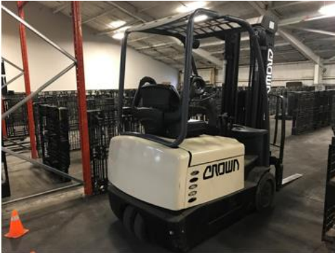
Class 1 – Electric Motor Rider Trucks (Operator Sits)
