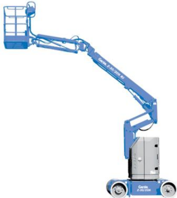
Type 3 (controlled from platform)
