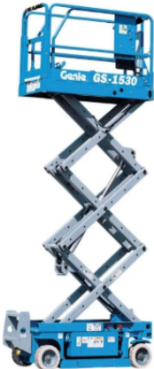
Type 3 (controlled from platform)
