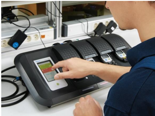
Bump test using a docking station.
