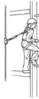
Example of a fall arrester in use on a vertical structure
