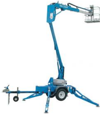
Type 1 (must be stowed to move)
