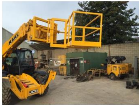
Type 2 (controlled from chassis)
