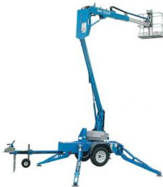
Type 1 (must be stowed to move)
