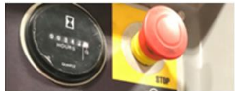
Lock-out emergency stop.
