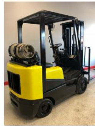
Class 4 – Internal Combustion Trucks – Cushion Tires Only (Operator Sits)
