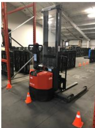
Class 3 – Electric Motor Hand Trucks (Operator Stands)
