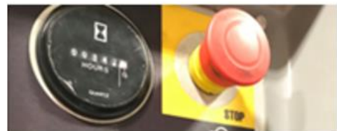
Lock-out emergency stop.
