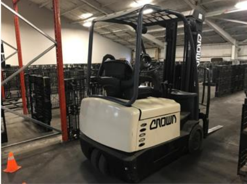
Class 1 – Electric Motor Rider Trucks (Operator Sits)
