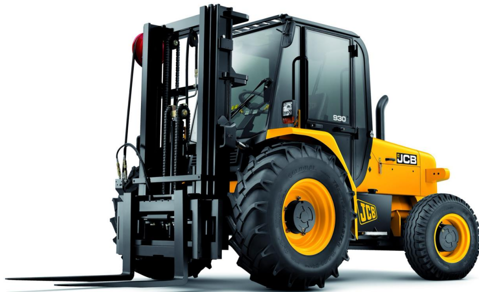
Class 7 – Rough Terrain Forklift Trucks (Operator Sits)
