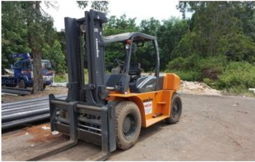
Class 5 – Internal Combustion Trucks – Pneumatic Tires Only (Operator Sits)
