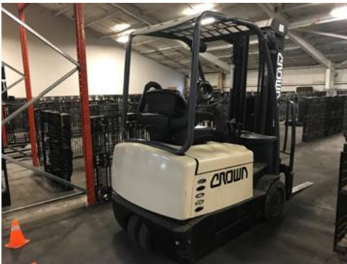
Class 1 – Electric Motor Rider Trucks (Operator Sits)
