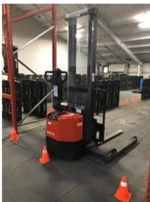
Class 3 – Electric Motor Hand Trucks (Operator Stands)
