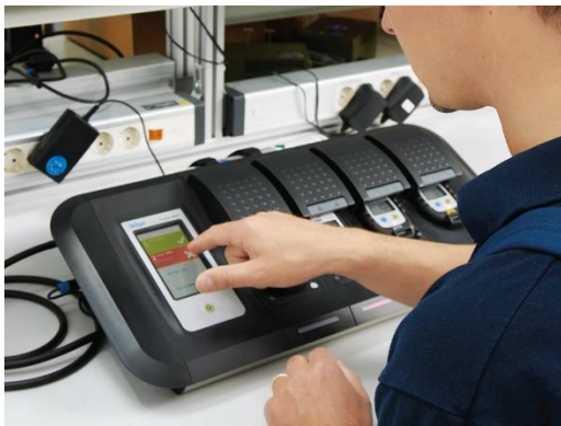
Bump test using a docking station.
