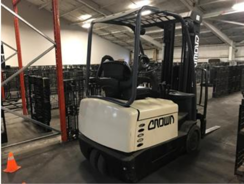
Class 1 – Electric Motor Rider Trucks (Operator Sits)
