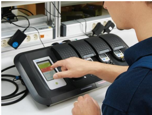
Bump test using a docking station.
