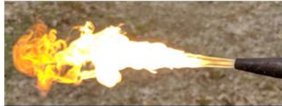
This is an oxy-acetylene torch flame BEFORE the oxygen is turned on.
