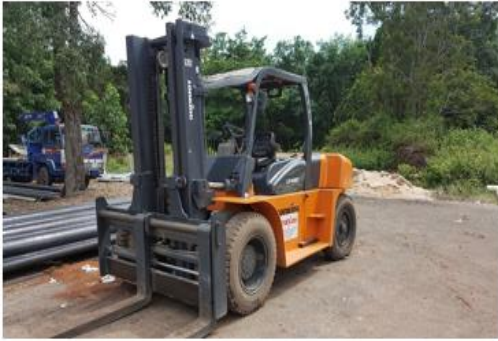
Class 5 – Internal Combustion Trucks – Pneumatic Tires Only (Operator Sits)
