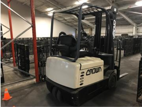
Class 1 – Electric Motor Rider Trucks (Operator Sits)
