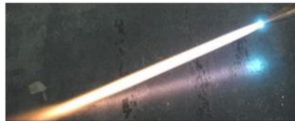
This is an oxy-acetylene torch flame AFTER the oxygen is turned on.
