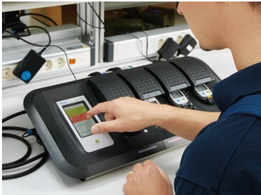
Bump test using a docking station.
