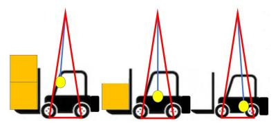
Operators need to consider the effect of leverage upon their equipment while lifting and carrying loads.
