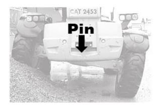
Because the rear axle oscillates, it is less stable than the front axle.
