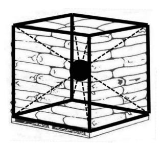
The operator needs to distinguish the centre of the load from the centre of gravity of the load.
