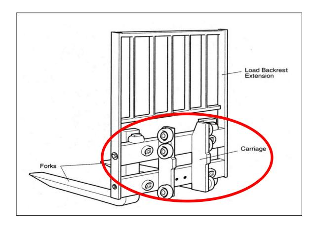
The carriage provides the connection between the load carrying devices (Forks) and the lifting device (Mast or boom).
