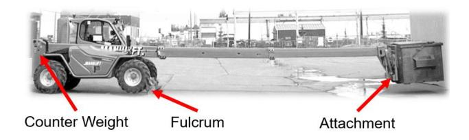
For machines intended to lift and carry load, the purpose of a counterweight is to offset the potential load to be carried.
