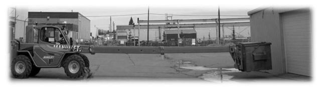
If the machine were to ever become loaded beyond capacity, the likelihood of the machine tipping forward increases.
