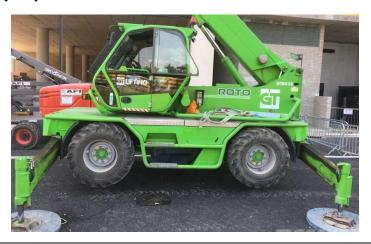
Note the outrigger pads being used on this VRLT. Always a good idea, a must if ground stability is unknown.
