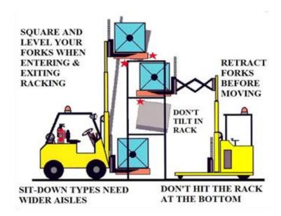
Keep in mind that racks should be designed and built for the intended capacities.
