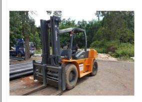
Class 5 – Internal Combustion Trucks – Pneumatic Tires Only (Operator Sits)
