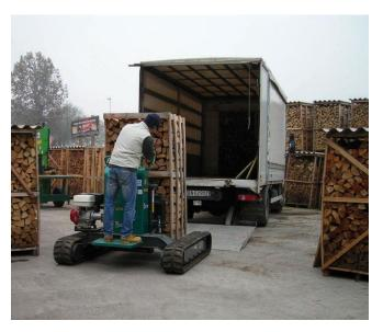
• Tracks are very aggressive while ascending and descending inclines but are significantly less aggressive on side slopes.
