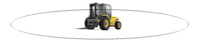
The above image represents the machines safe operating zone. This concept would be applied to any lift truck as a company policy.
