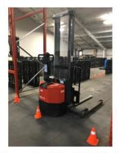
Class 3 – Electric Motor Hand Trucks (Operator Stands)
