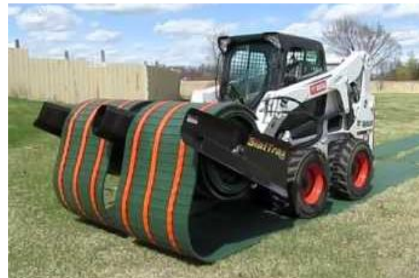
Note this skid-steer is laying turf protection.
