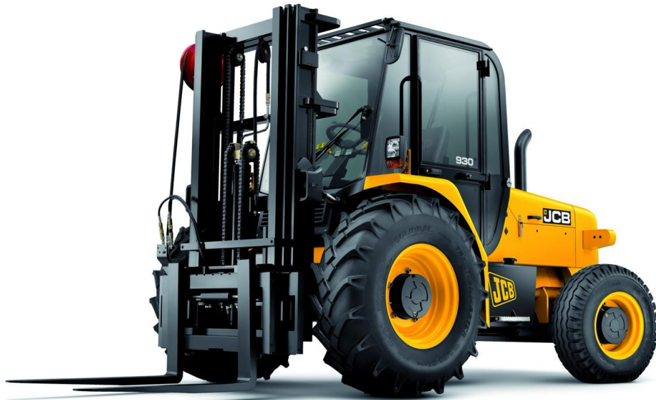
Class 7 – Rough Terrain Forklift Trucks (Operator Sits)
