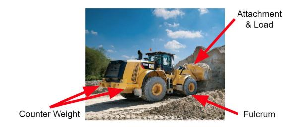
On level ground, 70% of the machines centre of gravity sits over the rear fulcrum due to the counterweight.
