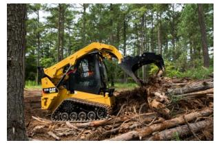
Skid steer: Available as a crawler or fourwheel-drive machine, skid steer loaders feature a unique lift-arm design and sturdy, rigid frame to deliver exceptional power in a small package. Skid steers are used in agriculture, construction, landscaping, road work and many other industries that benefit from its efficiency and versatility switching between work tools and attachments.
