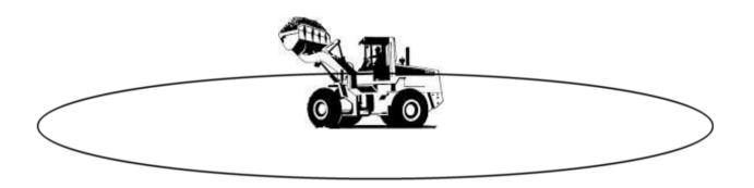
The above image represents the machines safe operating zone. This concept would be applied to any Mobile Equipment as a company policy.
