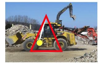
A raised load will cause the centre of gravity to shift even more toward the front.
