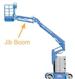
The jib is an extension from the primary/main boom that can be adjusted hydraulically.
