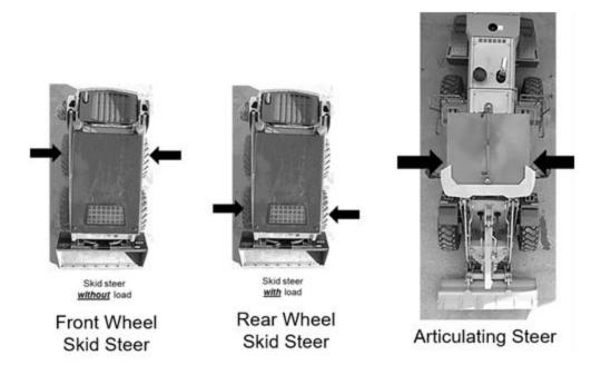
For equipment intended to lift and carry load at the front end of the equipment, manufacturers design the equipment with a steering mode that does not include the use of the front wheels for steering; for this type of equipment manufacturers avoid putting the heavy load over the steering axle to avoid damage that could occur to the steering mechanisms caused by the heavy load the equipment is carrying.
