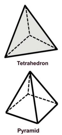
If the machine has four points of contact with the ground plus a point located near the top of the load at maximum height, we're essentially looking at the shape of a pyramid.
