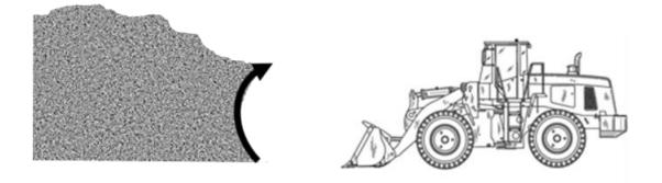
Using the arc penetration method, the bucket is forced into the pile and lifted upwards simultaneously in an arc until the bucket is filled.
