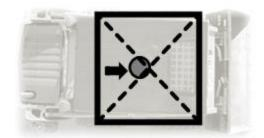
Because the center of gravity (depicted by the solid circle) lies within the stability tetrahedron, the machine remains within its range of stability.
