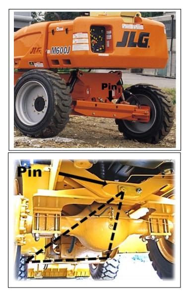
• Because the rear axle oscillates, it is less stable than the front axle.
