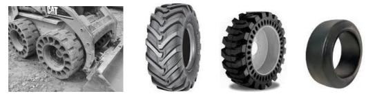
These "slicks" provide for a smoother, quieter ride with less vibration placed upon the machine and operator than those with tread, especially when used indoors.
