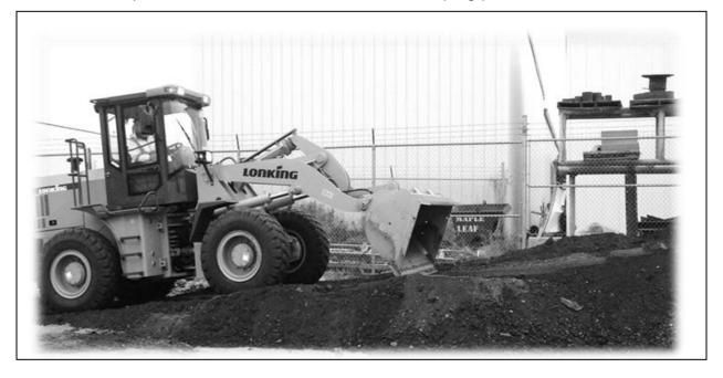
The detent position allows operators to drag material backwards into desired locations when building ramps and leveling areas; this is known as "back-dragging".
