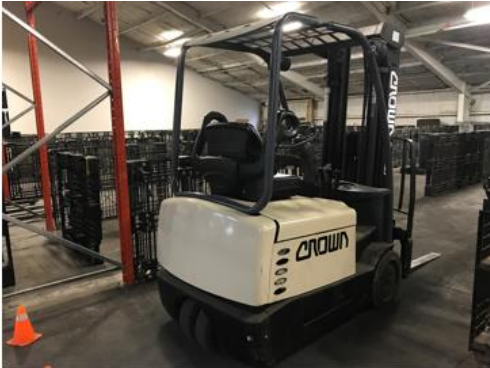
Class 1 – Electric Motor Rider Trucks (Operator Sits)
